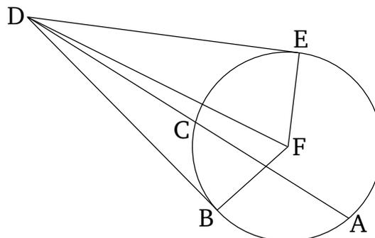
For let some point  $D$  have been taken outside circle  $ABC$ , and let two straight-lines,  $DCA$  and  $DB$ , radiate from  $D$  towards circle  $ABC$ , and let  $DCA$  cut the circle, and let  $DB$  meet (the circle). And let the (rectangle contained) by  $AD$  and  $DC$  be equal to the (square) on  $DB$ . I say that  $DB$  touches circle  $ABC$ .
