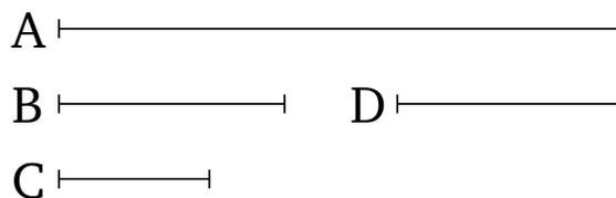
Let  $A, B$  and  $C$  be three proportional straight-lines, (such that) as  $A$  (is) to  $B$ , so  $B$  (is) to  $C$ . I say that the rectangle contained by  $A$  and  $C$  is equal to the square on  $B$ .
