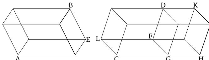
Let  $AB$  and  $CD$  be parallelepiped solids (having) the same height. I say that the parallelepiped solids  $AB$  and  $CD$  are to one another as their bases. That is to say, as base  $AE$  is to base  $CF$ , so solid  $AB$  (is) to solid  $CD$ .
