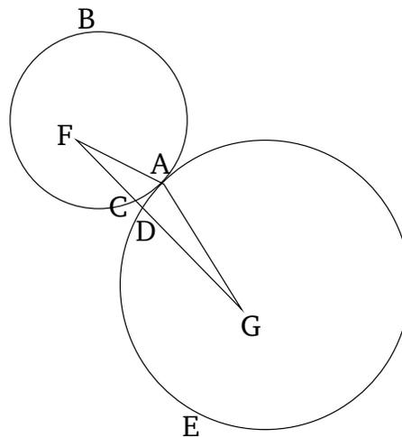
For let two circles,  $ABC$  and  $ADE$ , touch one another externally at point  $A$ , and let the center  $F$  of  $ABC$  have been found [Prop. 3.1], and (the center)  $G$  of  $ADE$  [Prop. 3.1]. I say that the straight-line joining  $F$  to  $G$  will go through the point of union at  $A$ .
