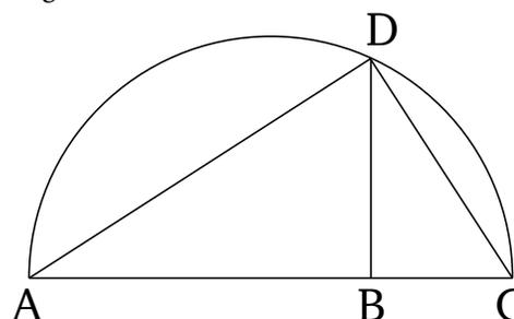
Let  $AB$  and  $BC$  be the two given straight-lines. So it is required to find the (straight-line) in mean proportion to  $AB$  and  $BC$ .
