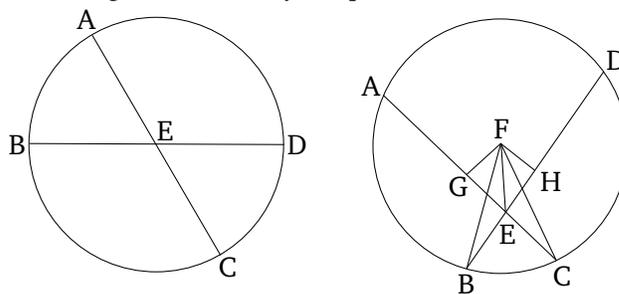
For let the two straight-lines  $AC$  and  $BD$ , in the circle  $ABCD$ , cut one another at point  $E$ . I say that the rectangle contained by  $AE$  and  $EC$  is equal to the rectangle contained by  $DE$  and  $EB$ .
